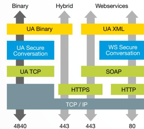
The OPC Foundation provides protocol implementations in the form of communication stacks written in three (3) different programming languages to its members, ANSI C, C# and Java. The stacks are maintained by the OPC Foundation to insure interoperability. Each stack provides a language specific API, the service encoding layer (binary or XML), the secure channel layer and the transport layer.
